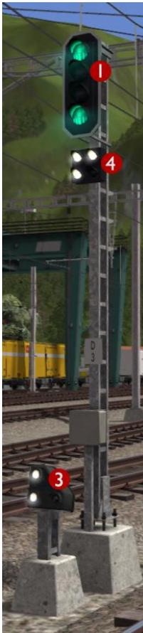
This is a main signal (Hauptsignal) that is currently showing Aspect 3 to alert the driver that 45 km/h is the maximum permissible speed allowed beyond this point.
