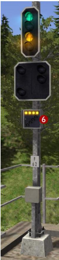
This combined signal on approach to a station has an additional Occupied Track Indicator.
