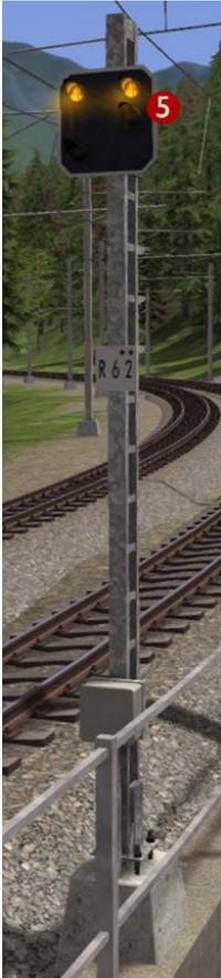
This is a Distant Repeater Signal that is currently showing that the next signal ahead is displaying Aspect 0 (Stop).
