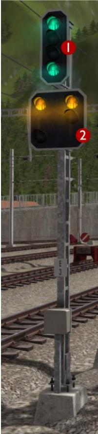
This is a combined signal that is currently showing Aspect 3 on the Main Signal Head to alert the driver that 45 km/h is the maximum permissible speed allowed beyond this point. The Distant Signal Head is showing that the next signal ahead is displaying Aspect 0 (Stop).
