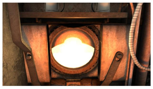
Figure 3. Fire is now an incandescent mass and the firebox has attained a creamy white colour.
