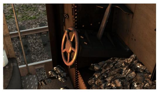
The hand brake is used to manually apply the brakes on the tender, it can be used to assist in gradually buffering up an unfitted train. However, it is not a very powerful brake and so the vacuum brake will need to be used to assist in stopping long trains. It can be applied using the '*I*' key and released with '**Shift** + *I*'.
