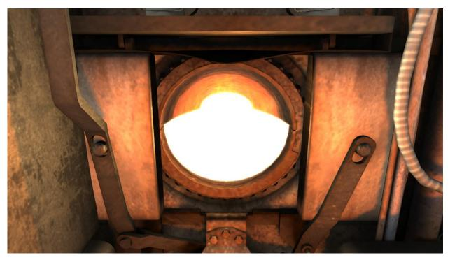
Figure 4. Both the fire and the firebox are incandescent white and it is practically impossible to distinguish where the fire bed is.
