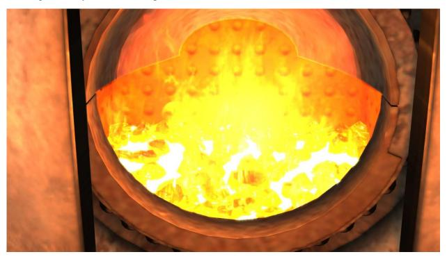
In the above picture, the fire is at the ideal fire mass, the coals should just cover the row of stay heads. As the fire mass drops the stay heads become much more visible and below around 360lb fire mass the firebars can begin to be seen.
