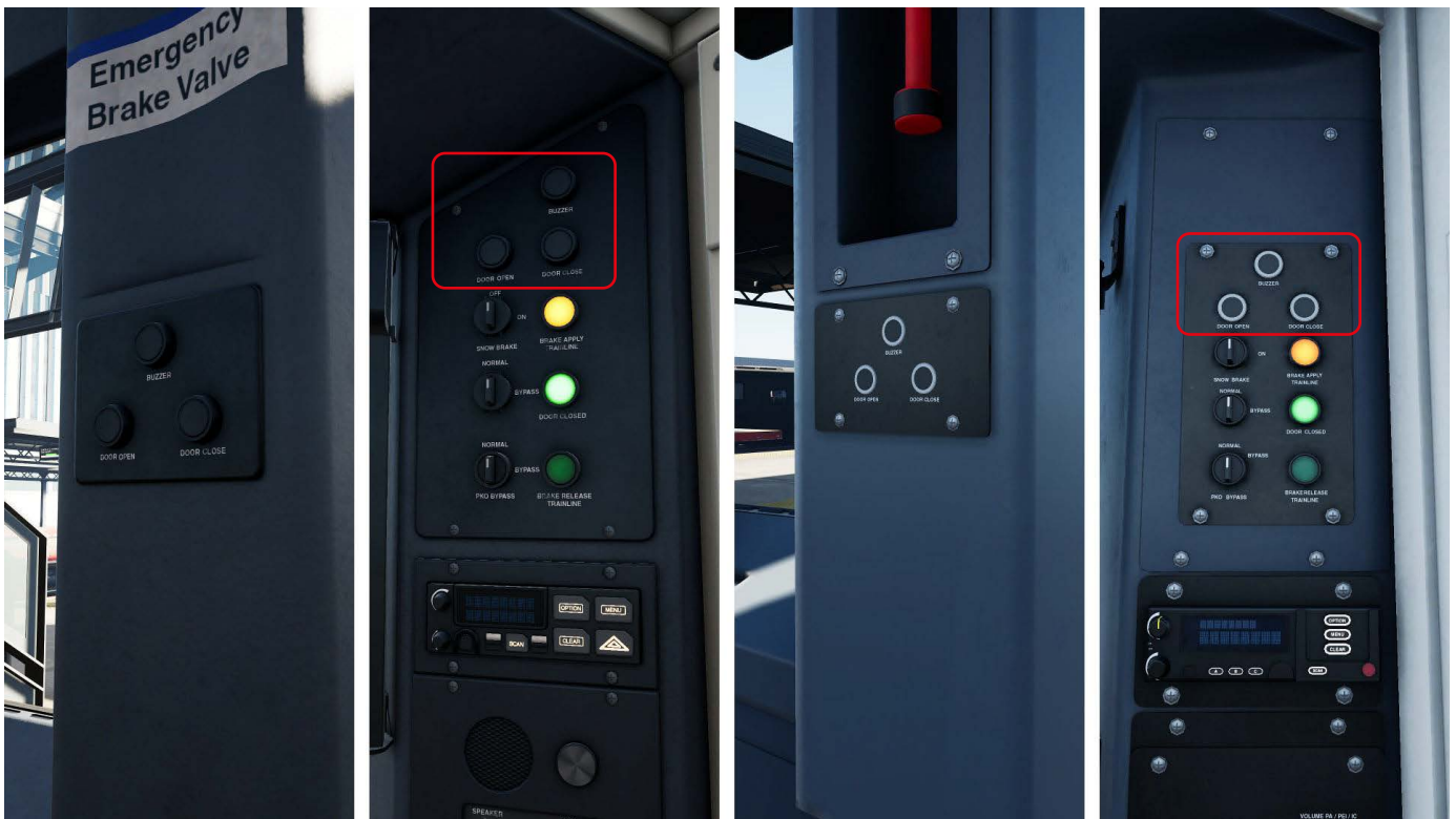
M7 left-side door controls | M7 right-side door controls | M9 left-side door controls | M9 right-side door controls
