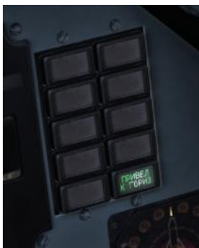
Figure 44: "ПРИВЕД К ГОРИЗ" (Level to the horizon) annunciator
