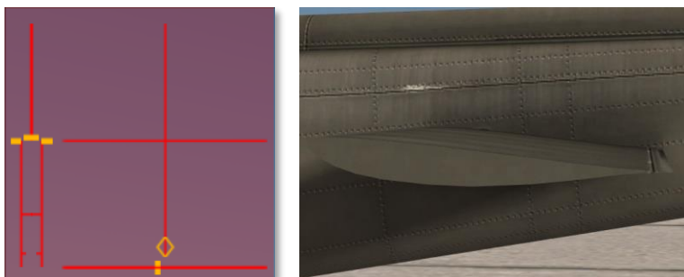
Figure 4.4. Position of the synchronized elevator when cyclic is fully back (angle +1.28 degrees).
