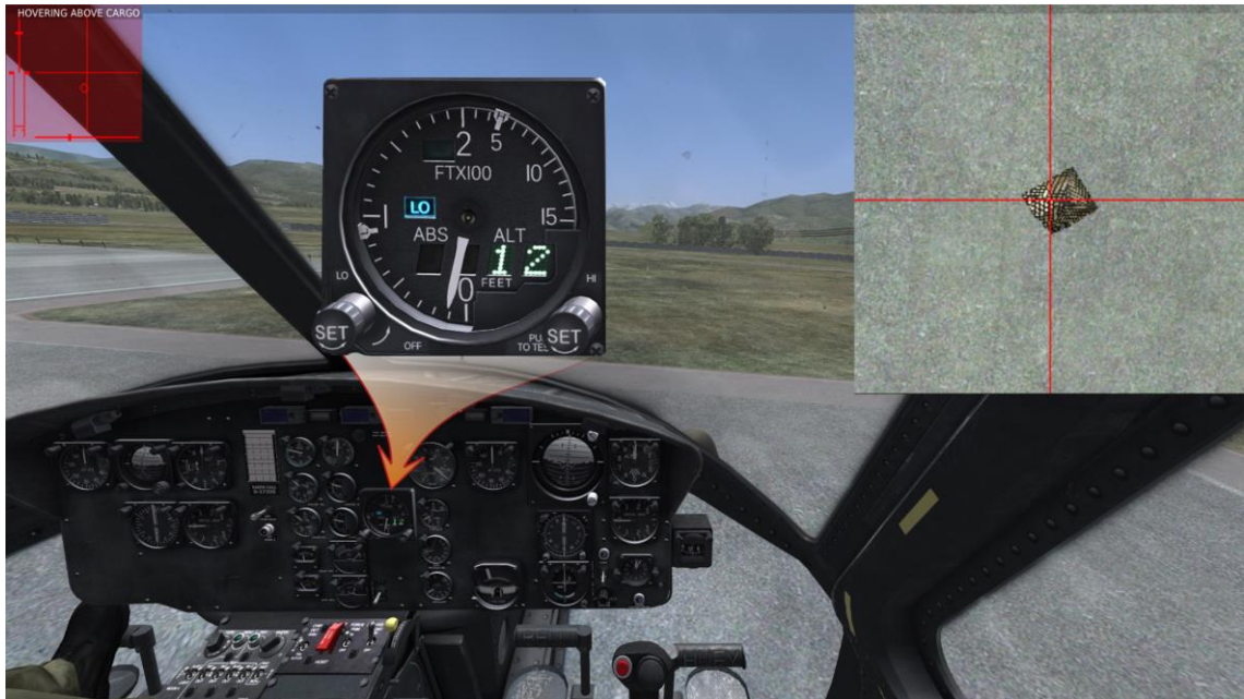
Figure 11.7. Conditions for Automatic Attachment of Load at Hovering Method (1 of 2).
