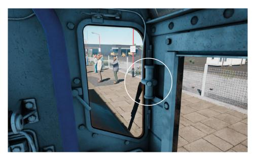
Use the button on the wiper motors to operate the windscreen wipers. They are variable speed.
