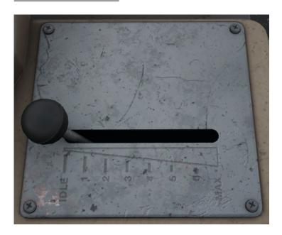
Moving the lever backwards will increase the engine RPM from IDLE to MAX through six intermediate stages.
