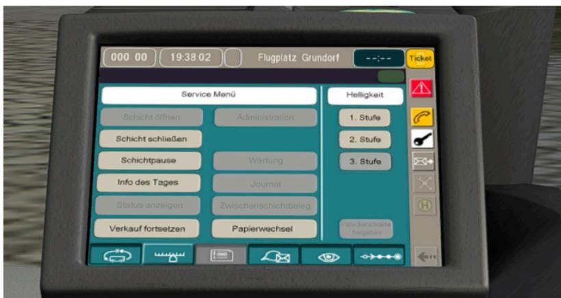
The settings mode allows for the shift to be paused or terminated. The screen brightness can also be changed here. The device has a selection menu to the right. Clicking on the yellow icon on the upper right-hand corner switches the device from "IBIS mode" to "selling mode". In the center of the screen the type of ticket can be changed.
