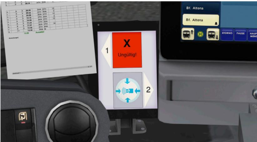
The driver check display is installed between the dashboard and the ticket printer. You will see the scan result of each passenger passing by and scanning their ticket. You can also click both of the boxes on the screen to disable the corresponding terminal for scanning.
