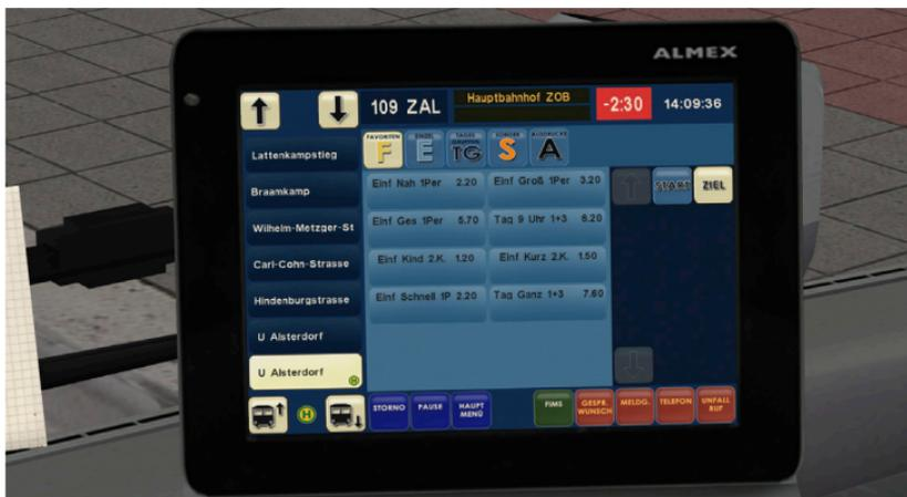
The ALMEX ticket printer ("EFAD 2") is a highly advanced touchscreen device that was developed in cooperation with HOCHBAHN. It sells tickets, controls the target display, interior stop display and plays station announcements.
