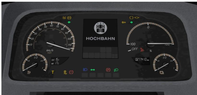
In contrast to the older monochromatic and well-arranged displays, a new small colored display was introduced. There are several check lights scattered over the panel, while some icons are also shown in the display.
