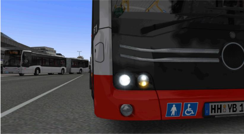
The exterior lights are mainly based on LED technology. This bus features a new automatic light control which is used by default when the light selector switch is set to "A". This mode will automatically toggle headlights and standing lights.
