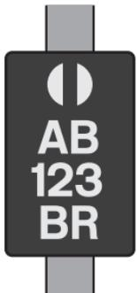
The upper part of the identification plate employs a form of code that advises the driver on what type of signal is deployed. In this instance, a three aspect banner repeater.
