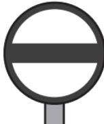
The horizontal band denotes the next main signal is displaying a stop aspect. You should be prepared to stop at the next signal.
