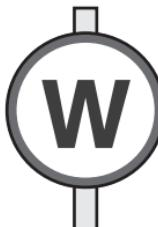
The modern variant of the whistle board at which the driver must make a clear single loud tone on the horn if between the hours of 7:30 am and 11:30 pm. At some sites, particularly at crossings it will be necessary to use a loud two-tone horn. Between the hours of 11:30 pm and 7:30 am, drivers must use discretion in use of the horn and should use a low tone except when required to warn other users of the railway of your approach, loud tones can therefore be used for this purpose.
