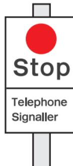
The Fixed Stop Board replaces the role of a controllable stop signal and essentially is regarded as a Stop aspect. You should stop at the board and then carry out the instructions indicated on the board before proceeding. In Train Sim World, the instructions are typically not simulated so, you may proceed beyond the board without carrying out the instructions advised.
