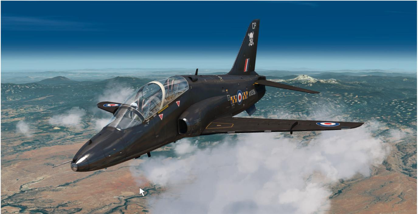
Aerodynamically, the aircraft is of conventional design with a moderately swept wing with a 2° dihedral and trailing edge double-slotted flaps. A one-piece all-moving tailplane is swept back and has a 10° anhedral.
