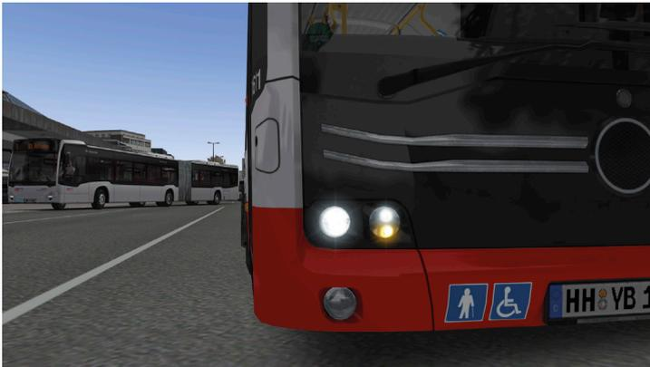
The exterior lights are mainly based on LED technology. This bus features a new automatic light control which is used by default when the light selector switch is set to "A". This mode will automatically toggle headlights and standing lights.
