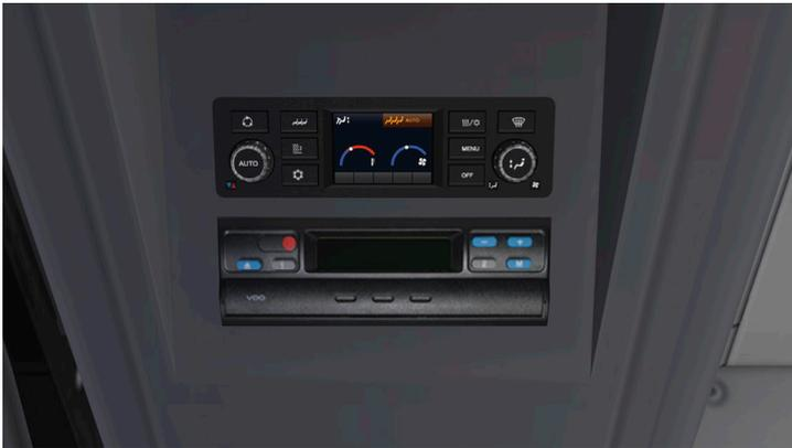
The saw tooth panels above the driver's place contain a digital trip recorder (not functional) and the A/C panel (see A/C control).
