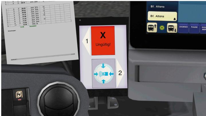
The driver check display is installed between the dashboard and the ticket printer. You will see the scan result of each passenger passing by and scanning their ticket. You can also click both of the boxes on the screen to disable the corresponding terminal for scanning.
