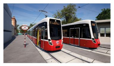
Shortly before the end of 2017, the prototype of the new Vienna tram was finished, and in 2018 it was delivered to Wiener Linien. The new low-floor trams are gradually replacing the remaining high-floor models. The Flexity is energy-efficient, featuring LED lighting and auto-adjusting air conditioning based on passenger numbers.
